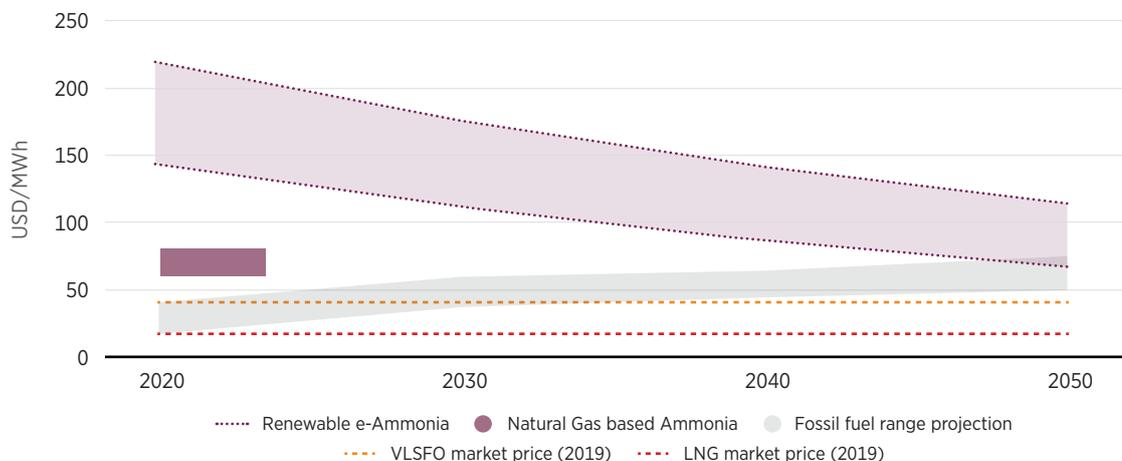
Note: Figure refers to the cost of fuel production. The total cost of ownership (e.g. machinery, storage and other) is not captured.
