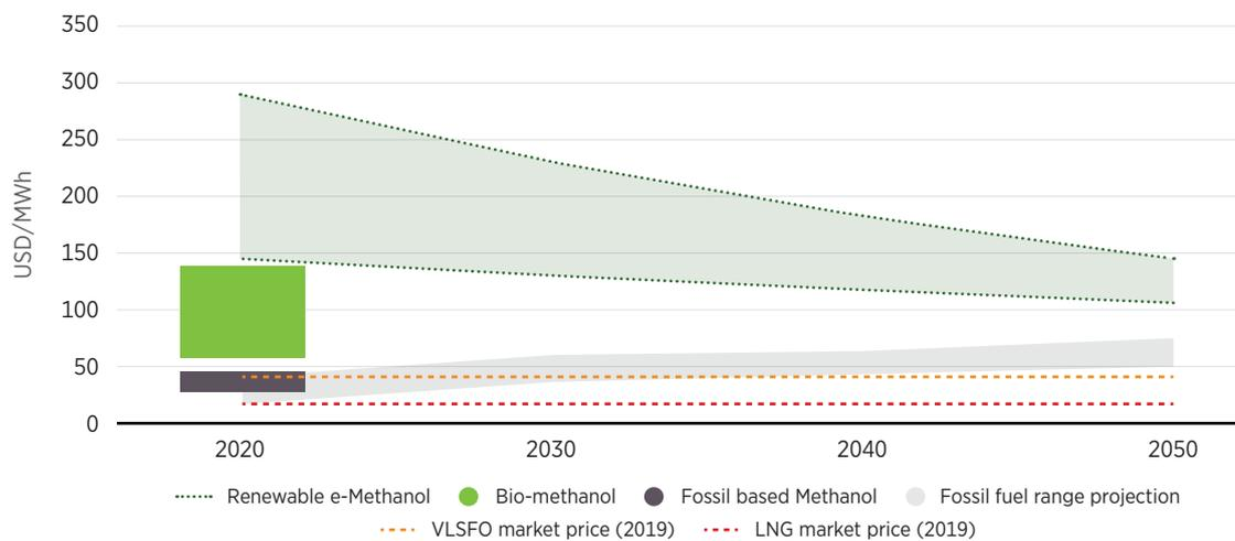
Note: Figure refers to the cost of fuel production. The total cost of ownership (*e.g.* machinery, storage and other) is not captured.
