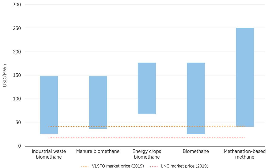
Note: Figure refers to the cost of fuel production. The total cost of ownership (e.g. machinery, storage and other) is not captured.
